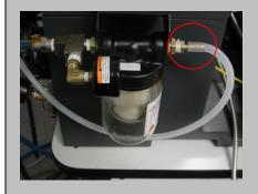
• Route the new site solder tube to the barb fitting on the filter jar as shown.
