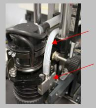
• Locate the site solder tube and remove it from the bracket.
