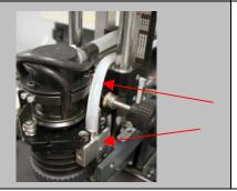
• Attach the new tube to the bracket, Verify the tube routing and reattach the nozzle heat shield.
