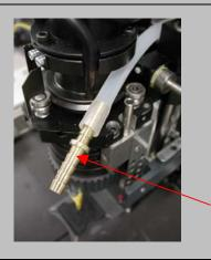
Install the double barb fitting into the existing site solder tube, as shown.
