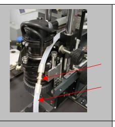
• Attach the new length of site solder tube (7') to the other end of the double barb fitting.
